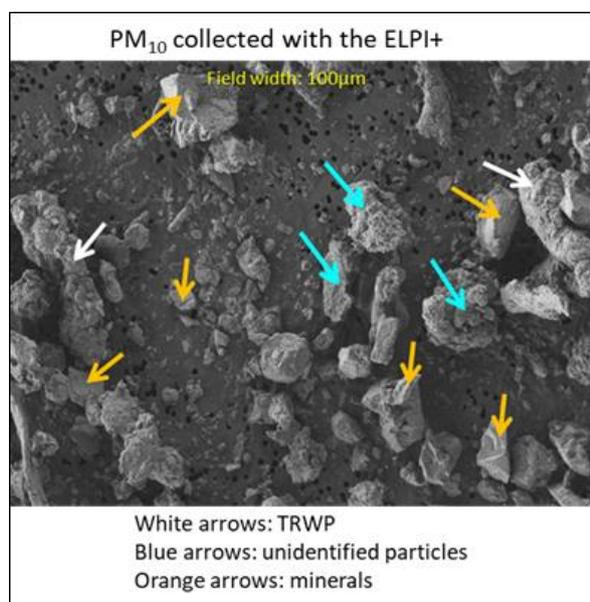
For PM<sub>2.5</sub>, no known morphology has been observed and it was not possible to identify TRWP among the particles collected. Brake particles have been collected directly on the brake disc and observed via microscopy. The morphology of brake particles is different from the one of TRWP and this seems to confirm that most of the PM<sub>2.5</sub> collected with the ELPI+ come from the brakes.
