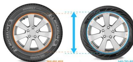
Michelin engineers designed an entirely new-sized tire (145/70 R 17) specifically for this concept car to provide it with outstanding aerodynamic qualities and energy efficiency.
