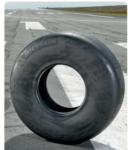
**The latest radial NZG technology tire for the Airbus A350**
